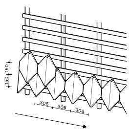
4. Continue with the next rows. Tiles can be cut to fit as necessary.
